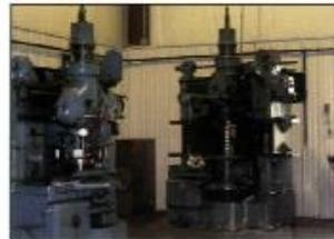
Gear Shapers cut internal and external gear teeth.
